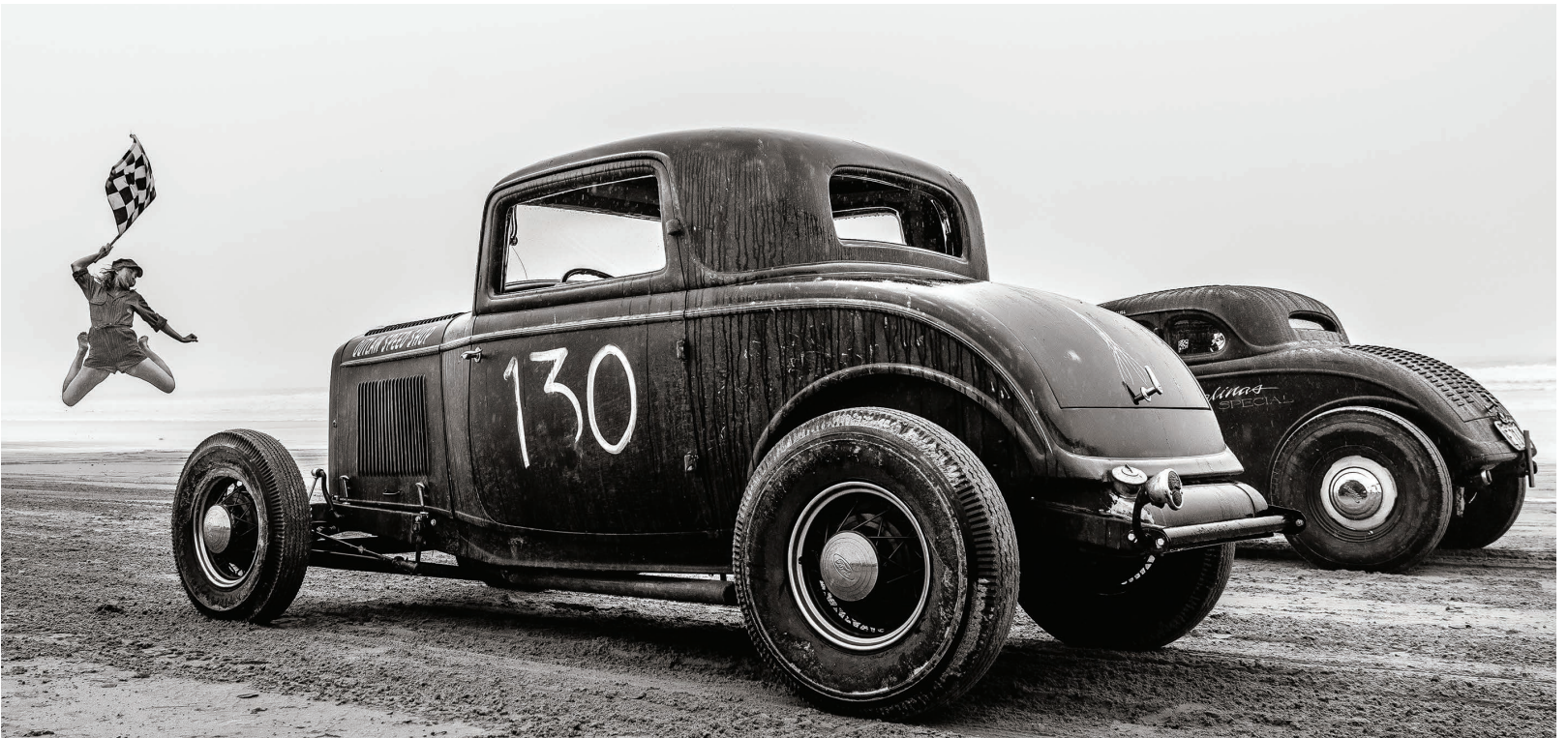
One of the more inventive TROG entries was raced by Oilers Car Club member Jeremy Baye of 1945 Speed and Custom. Jeremy combined a '22 Model T touring body, shortened '27 Essex frame and Ford flathead to create this mid-engined marvel. After thrashing to build the car in a matter of weeks, he made the mad dash to Pismo from his home in New York.
